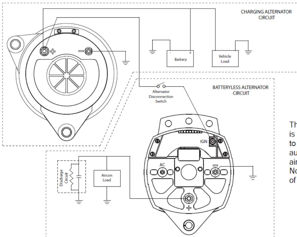
This type of alternator is used to supply power to operate fixed load auxiliary systems, eg. airconditioning. Note: Not for use as part of charging system .
